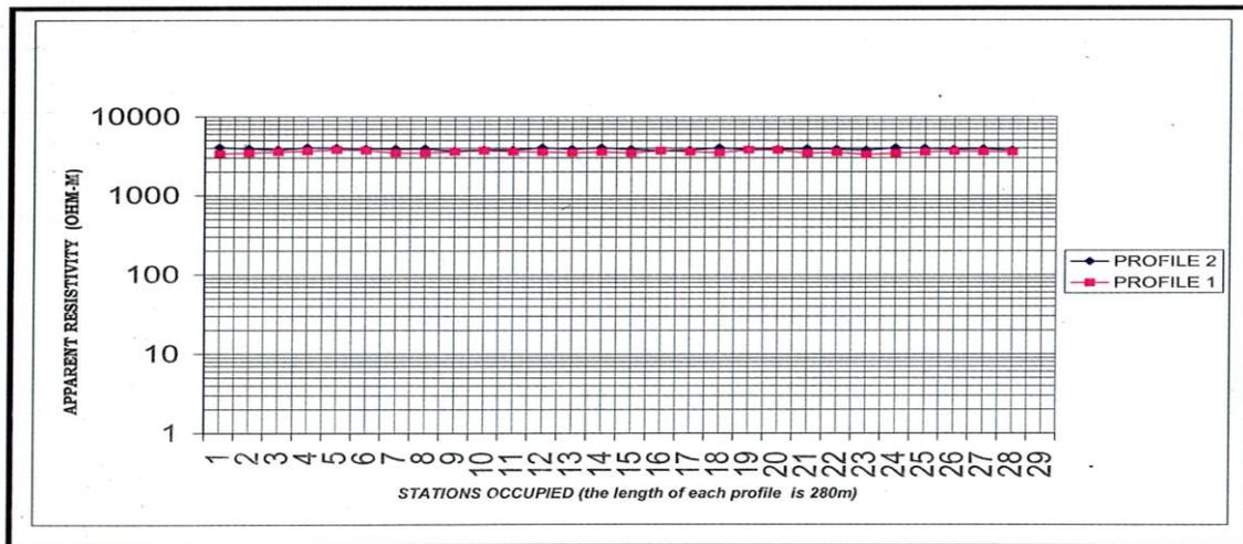
Figure 6a: The Wenner (CST) Traverse Curves beneath VES 1, VES 2 and VES 3 along Profile F1 and F2.
