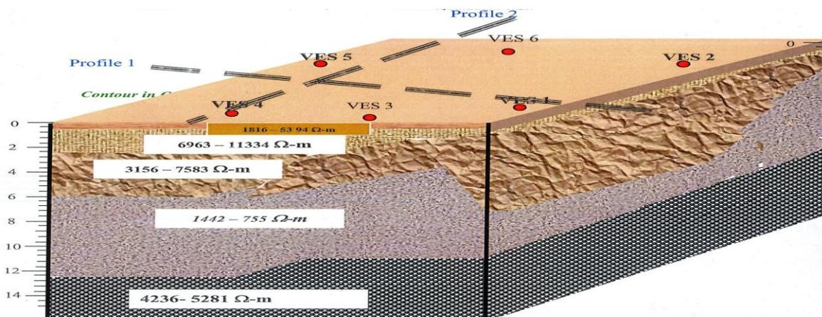
**Figure 7:** 3-D Geo-electric Model of the Surveyed Area
