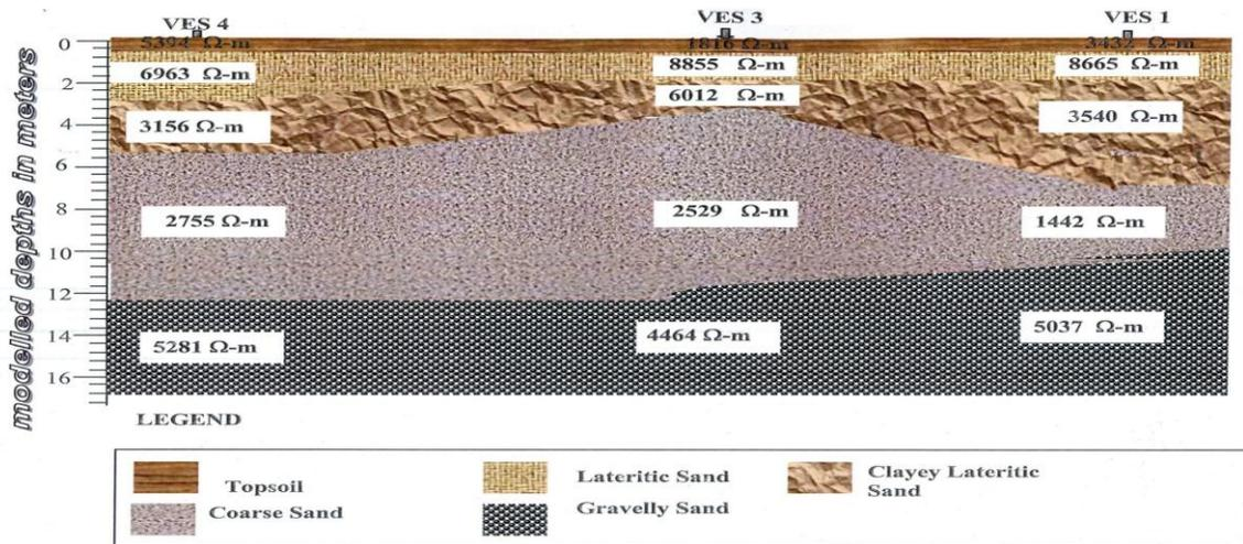
Figure 5b: 2-D Geo-electric section Beneath Transect BB' Connecting VES 4, VES 3 and VES 1
